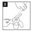
Place the shear pin in the appropriate hole within the drive shaft (1). Place the boat rotor on the drive shaft so that the shear pin engages in the slot in the back of the screw (2). When the screw is in place, install the stainless steel washer and locknut on the shaft.
